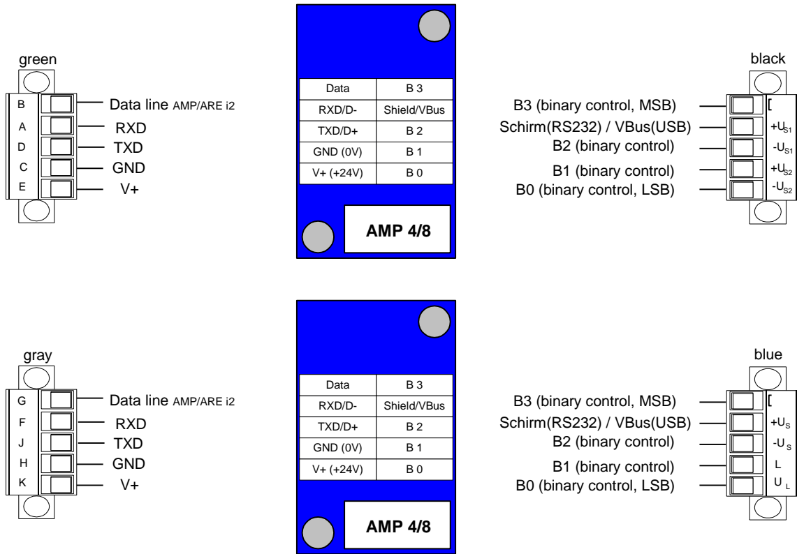
Figure 4: Pin assignment of the SAB connector
