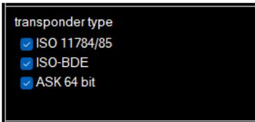
You can set any combination of the available transponder types to be read by checking the corresponding check boxes.
