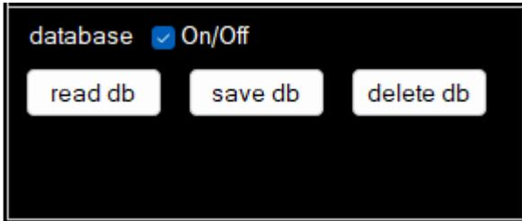
Some ARE H3.0 versions do contain a database functionality. This saves 2000 read transponder numbers including data, temperature, date and time where applicable.
