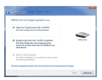
The pairing code "0000" must be entered in the input field of the following dialog box.
