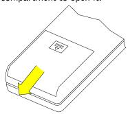
Attach the Battery to the connector inside. Put the Battery into the compartment.
