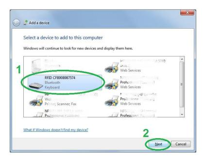
When the ARE H9 HF has been found, it has to be selected and then the "Next" button should be clicked to establish a connection to the ARE H9 HF.
