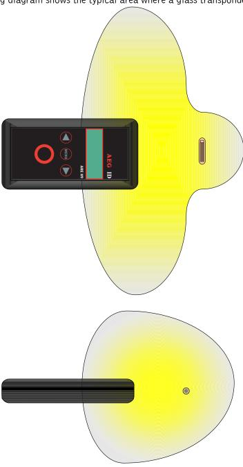
The ARE H 9 is not capable to read two or more transponders which are at the same time in the antenna field.
