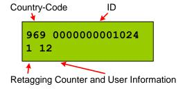
For ISO Transponder additional the retagging counter and the user information field are displayed in the second row of the display.
