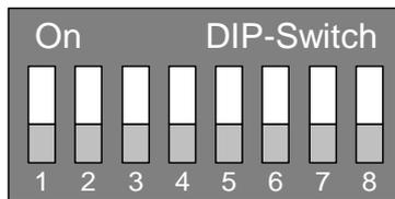
In normal condition (ex work) all DIP-switches are set OFF (down).
